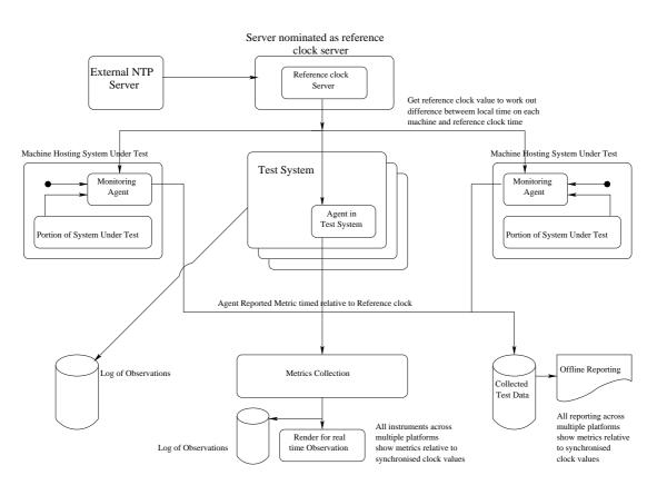
Figure 1: Overview of a System under Test using a Code Magus Limited Reference Clock implementation
