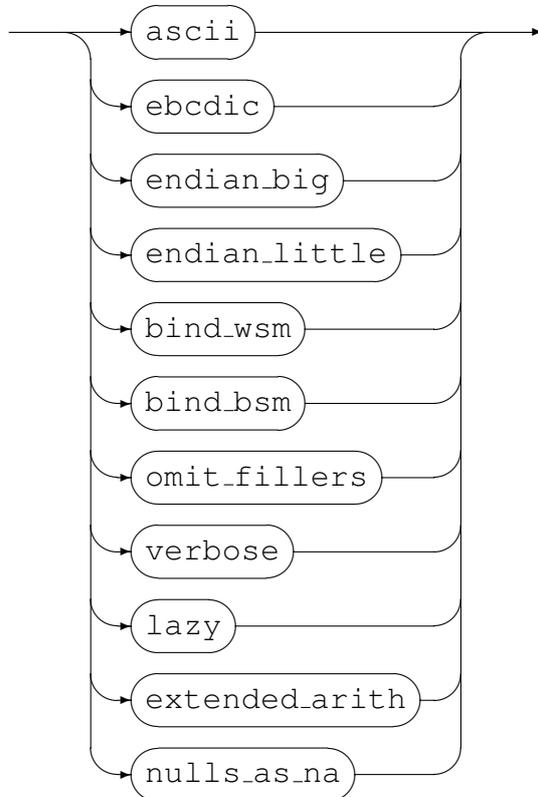
The *OptionsStatement* is used to supply meta-data attributes associated with the data which cannot be deduced from the meta-data (for in example from a COBOL copy-book), or which the local machine cannot be used as the default value for such attributes. Some of these options are also used to determine the manner in which the `objtypes` library component is to process the data.
